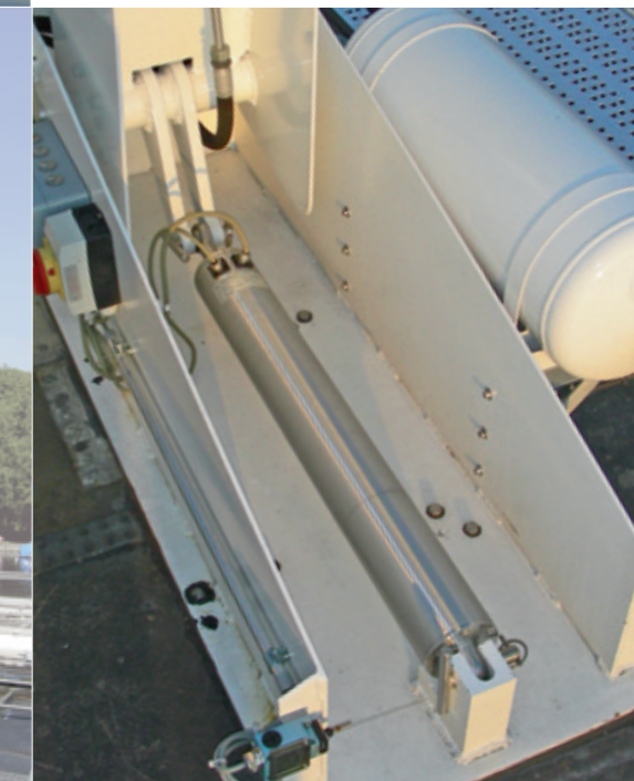
Linear actuator in "mast upright" operational position
